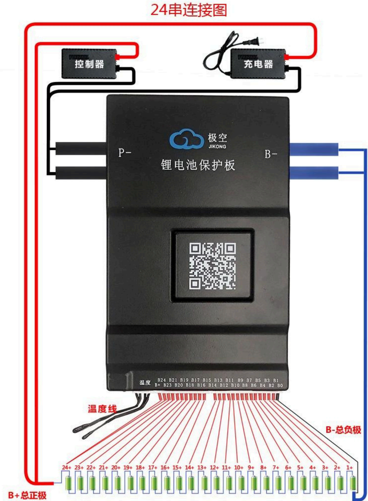
Figure 8 wiring diagram of 24 string batteries
