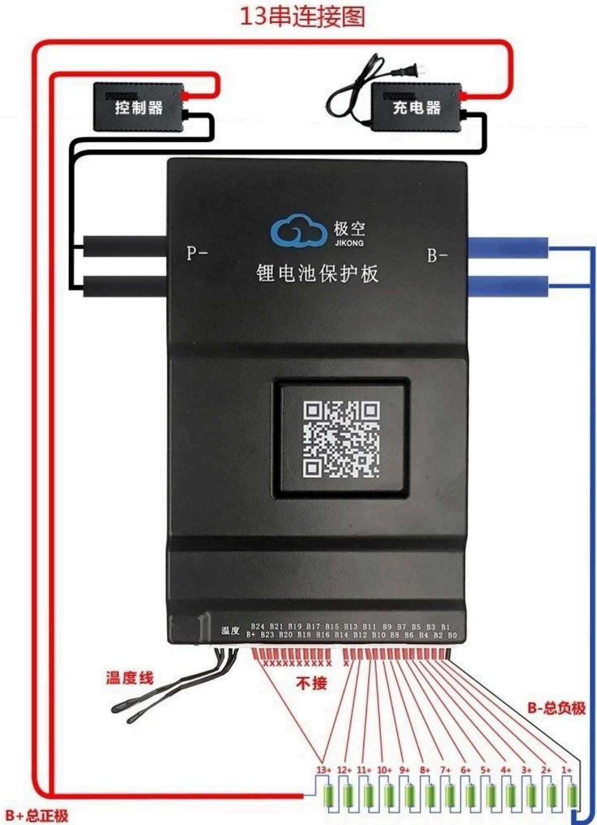
Figure 11 wiring diagram of 13 string batteries
